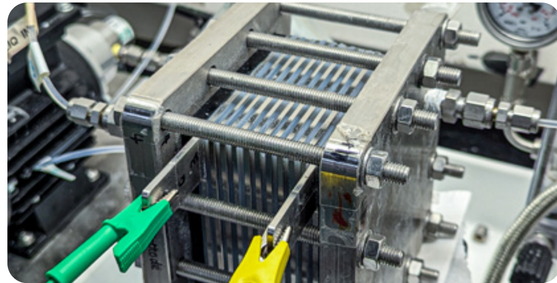
OzAmmonia's patented multiphase electrolyser
